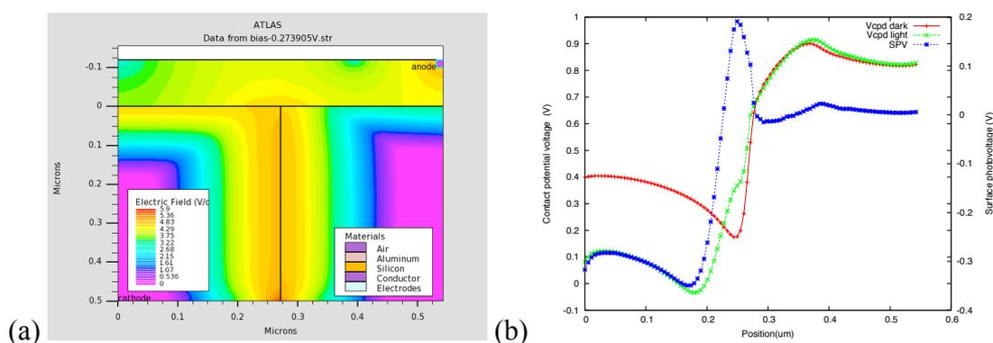
Figure 1 KPFM simulation showing (a) a silicon pn structure (b) a cross-sectional simulation of surface photovoltage which is the difference of light and dark contact potential voltages.
