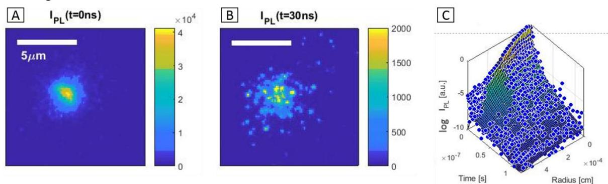
Figure (A) PL emitted by a CsPbI<sub>3</sub> quantum dot thin film 0 ns after being photo-excited ( $\lambda=532$  nm,  $5 \cdot 10^6$  photons/pulse). (B) PL emitted by the same sample 30 ns after the excitation. (C) time-resolved PL profiles in radial coordinates (blue circles) and fitted surface by the fitting algorithm.
